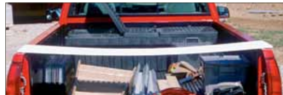
Ordinary soffits can't support their own weight over a long expanse.
